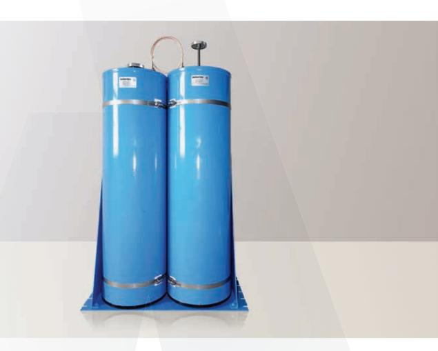
Mavitek MVD series band pass filters are designed and produced for the 117-138MHz band. MVD series cavity filters are made of blue enamel painted copper and housed in 19" rack mount. The connectors are silver plated and PTFE insulated. MVD series band pass filters can be ordered either in non-elongating tuning rod (MVD127P8NED2) or standard tuning rod configuration (MVD127P8D2)
